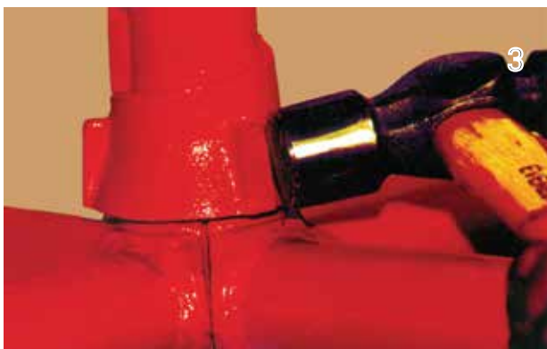
Rotate the top cup with hammer to lock the blade ends
